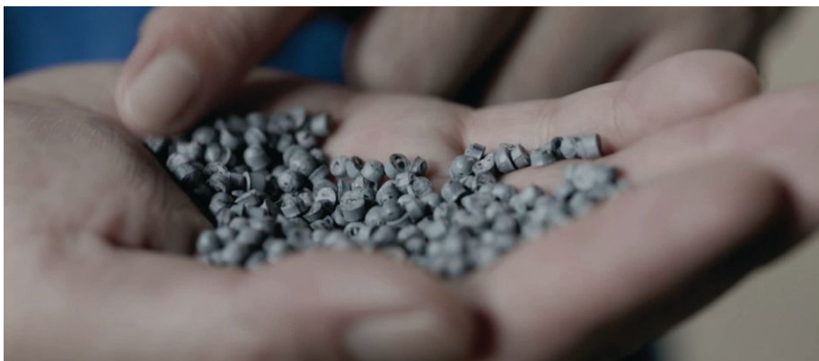
Thermoplastics are lightweight, averaging a weight of 1/16th of comparable metal materials.
