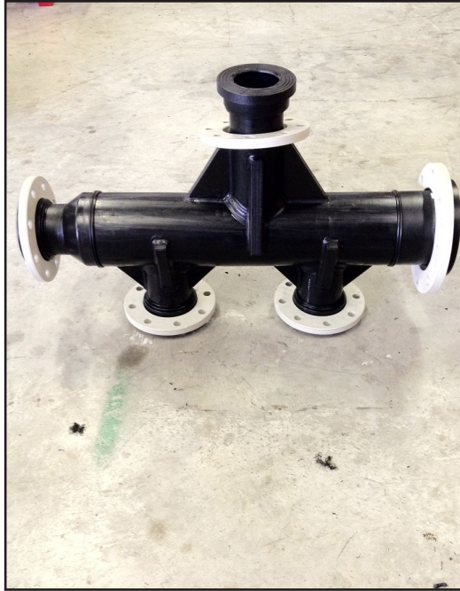
6" X 4" PUMP HEADER
